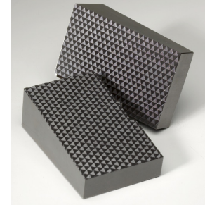
J1 Jaws (Flat specimens up to 2" wide x 1 1/2" thick)
