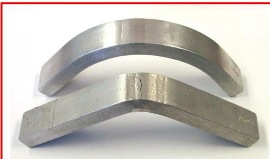
The specimen in front was tested in a standard guided bend tester and failed in weld metal. The specimen to the rear was tested in the wrap-around guided bend tester and was acceptable. In both test, the mandrel was 5 inch diameter (per MIS-22151, Aircraft and Missile Welding Operator's Qualification). Both specimens were removed from the same aluminum sample.
